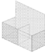
▲ Woven Mesh Gabions
